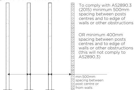
2. Drill holes in floor for location of anchor bolts
